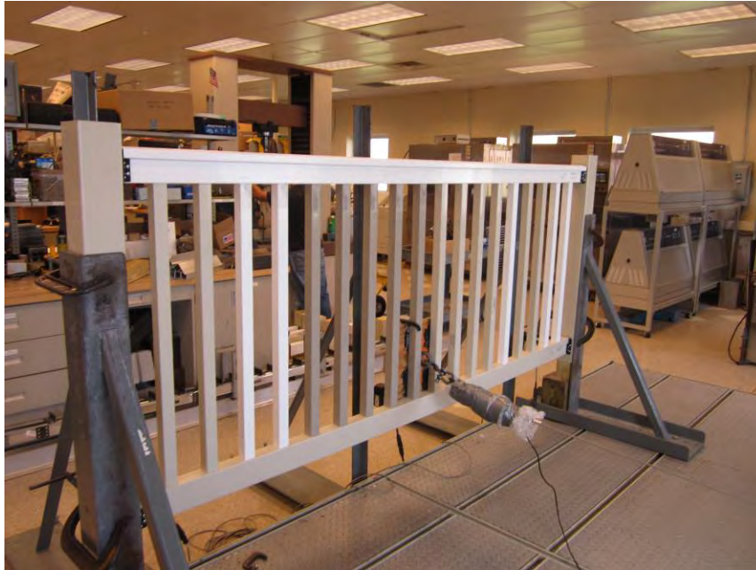
Photo No. 3 Infill Loading at Bottom of Two Balusters
