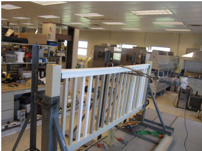
Photo No. 6 Concentrated Load at Midspan of Top Rail
