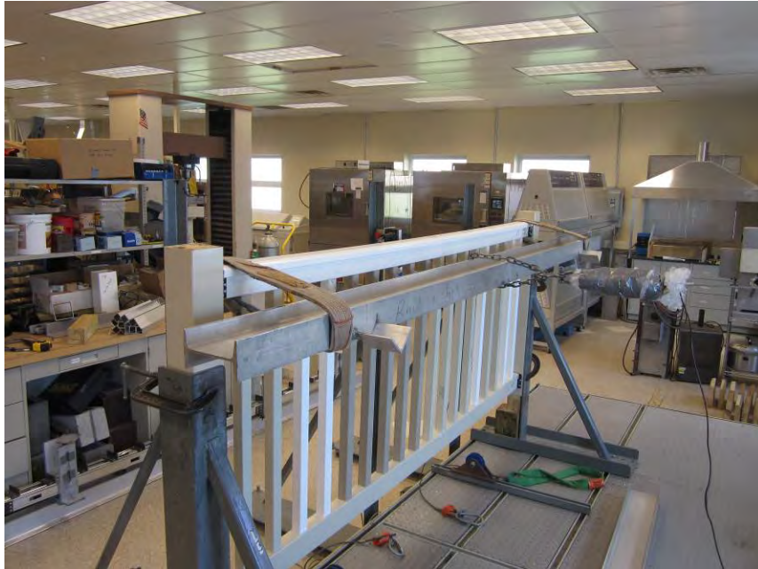
Photo No. 7 Concentrated Load at Both Ends of Top Rail (Brackets)
