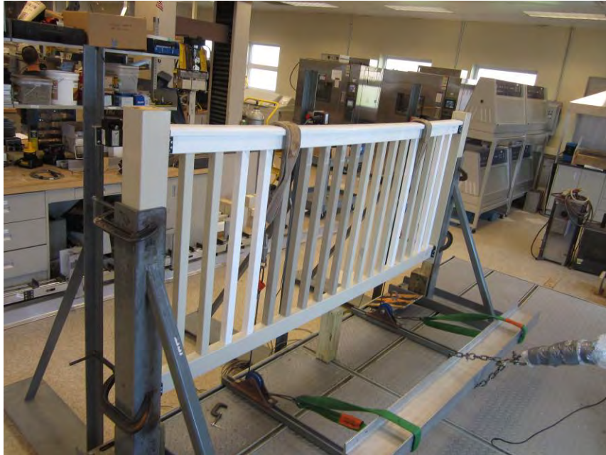
Photo No. 5 Vertical Uniform Load on Top Rail
